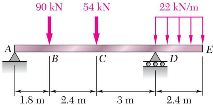
Draw the shear and bending moment diagrams for the beam and loading shown.
