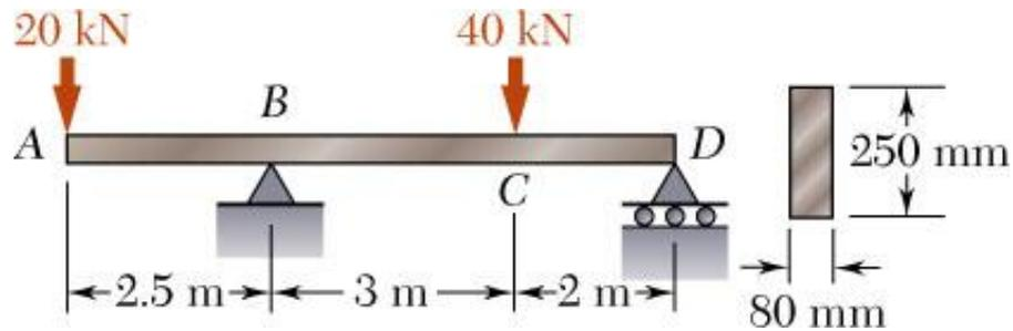
For the timber beam and loading shown, draw the shear and bending-moment diagrams and determine the maximum normal stress due to bending.
