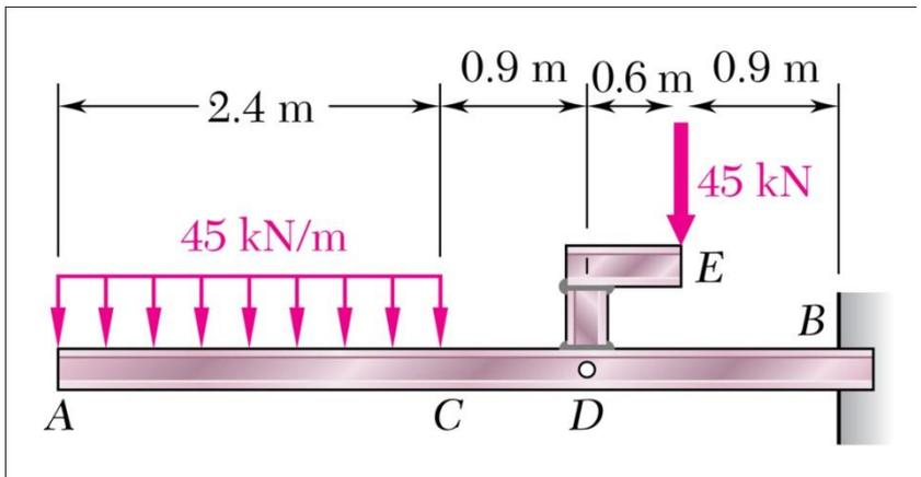
The structure shown is constructed of a W 250x167 rolled-steel beam. (a) Draw the shear and bending-moment diagrams for the beam and the given loading. (b) determine normal stress in sections just to the right and left of point *D*.
