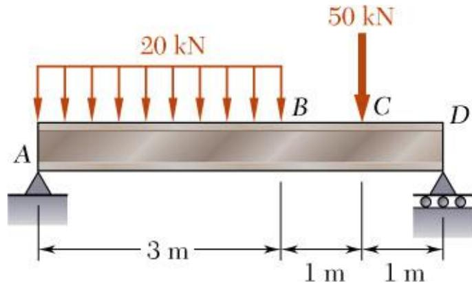
A simply supported steel beam is to carry the distributed and concentrated loads shown. Knowing that the allowable normal stress for the grade of steel to be used is 160 MPa, select the wide-flange shape that should be used.
