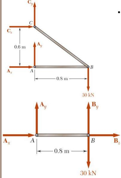
• In addition to the complete structure, each component must satisfy the conditions for static equilibrium
