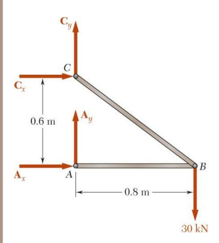
• Structure is detached from supports and the loads and reaction forces are indicated
