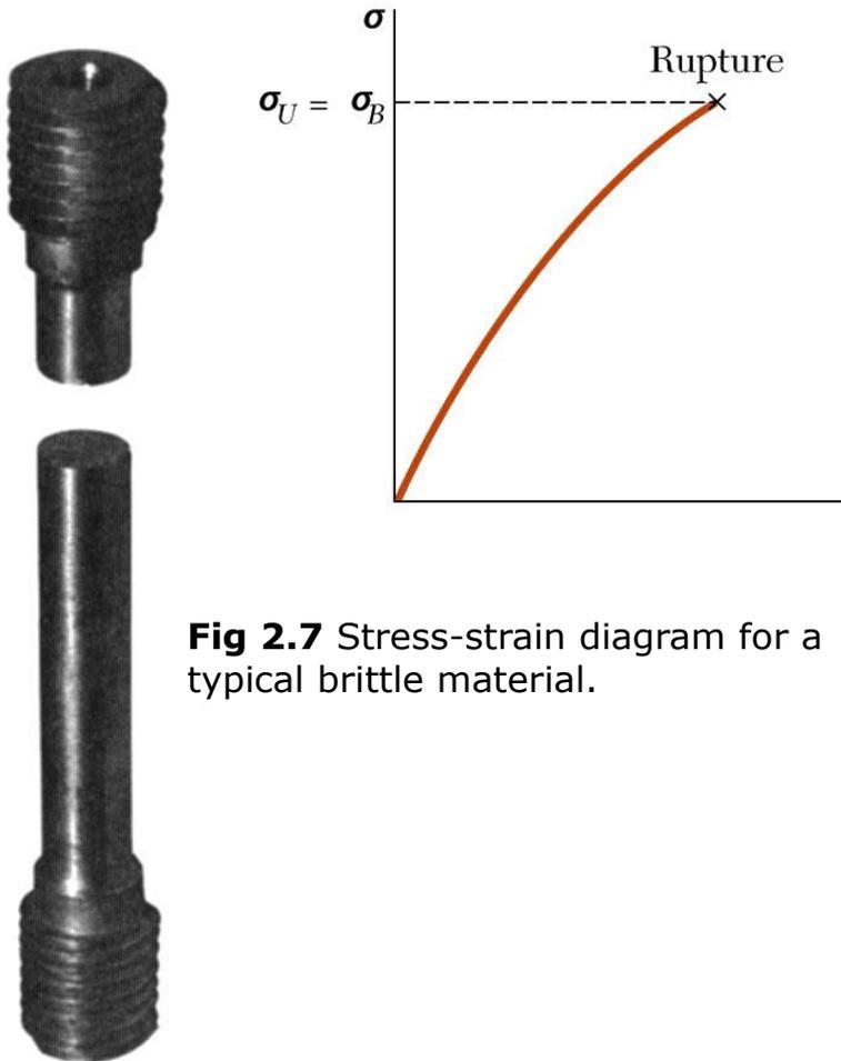
**Fig 2.7** Stress-strain diagram for a typical brittle material.
