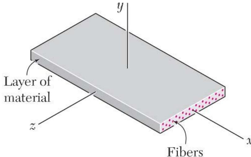
**Fig. 2.12** Layer of fiber-reinforced composite material.
