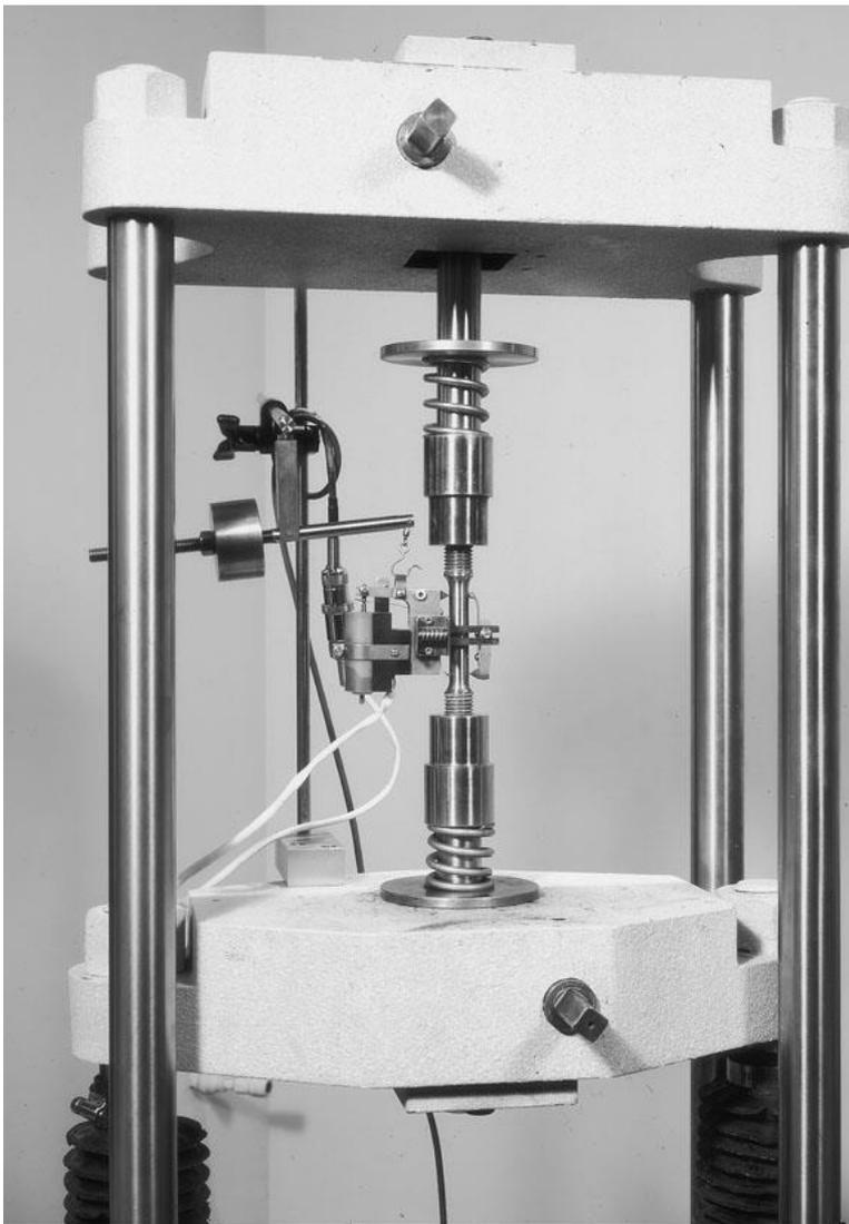
This machine is used to test tensile test specimens, such as those shown in this chapter.
