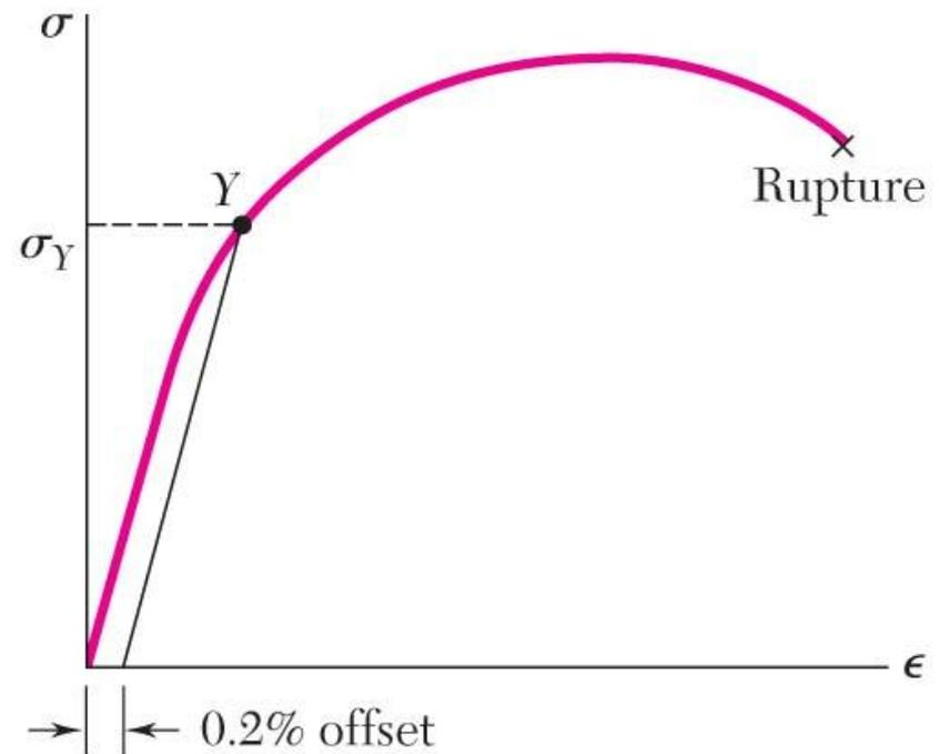
**Fig. 2.8** Determination of yield strength by offset method.
